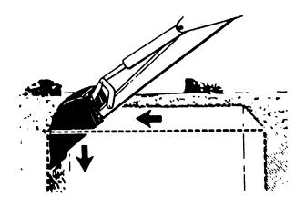
To finish the near wall, lift up and crowd in. Keep the edges of the bucket horizontal.
